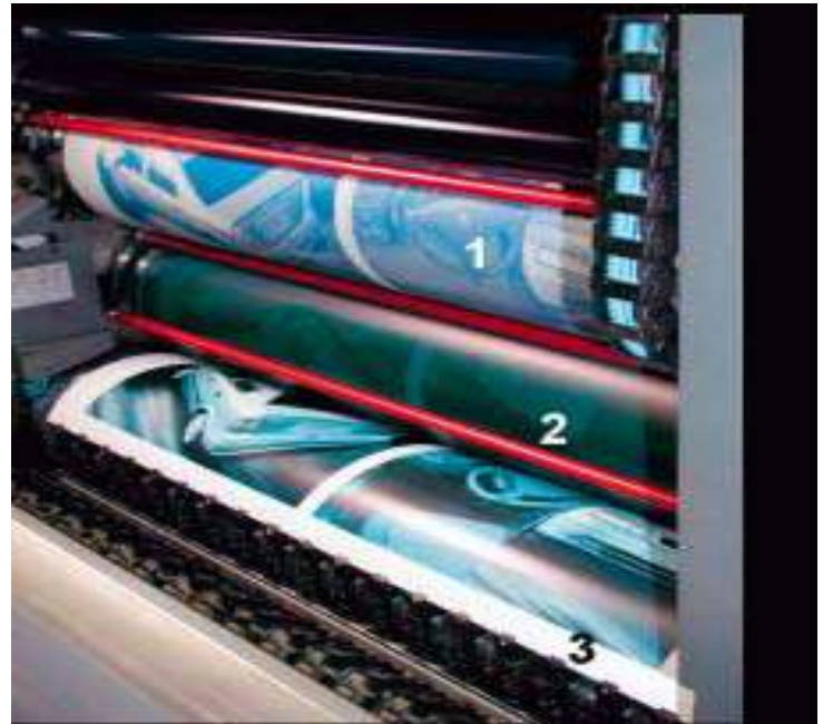
Printing unit with printed sheet on the impression cylinder: 1 Plate cylinder 2 Blanket cylinders 3 Impression cylinders with a printed sheet
