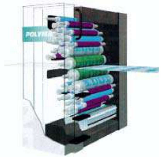
Double sided printing in a printing unit
